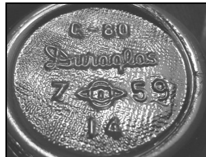
Figure 11 – Peened date code (eBay)
