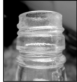
Figure 5c-38 – Finish for roll-on tamperproof cap; quart bottle
